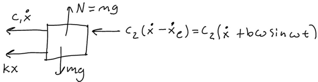
$$\rightarrow: -kx - c_1 \dot{x} - c_2(\dot{x} + b\omega \sin \omega t) = m\ddot{x}$$
