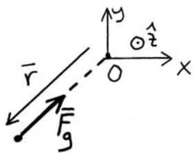
$$\overline{M}_{\mathcal{O}} \stackrel{(7.2)}{=} \overline{r} \times \overline{F}_g = \overline{0}$$
