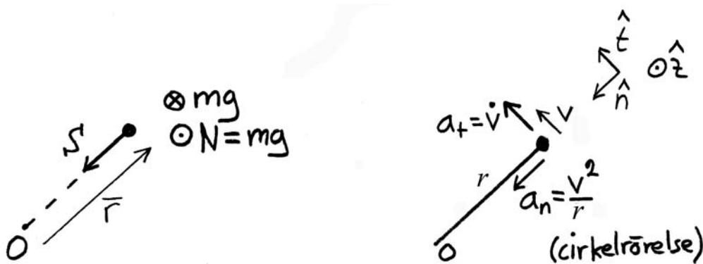
$$\overline{M}_{\mathcal{O}} = \overline{r} \times \overline{S} = \overline{0}$$
